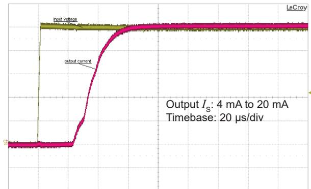
Figure 6: Typical delay time (0 to  $U_{PN}$ )
