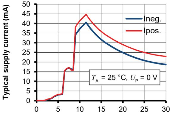
Figure 7: Supply current function of supply voltage
