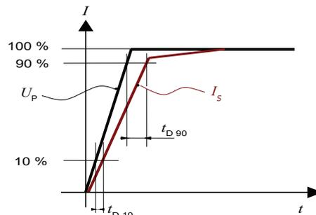
Figure 14: Delay time  $t_{D10}$  @ 10 % and delay time  $t_{D90}$  @ 90 %
