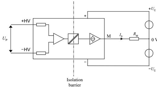
Figure 13: Standard characterization schematics for current output transducers ( $R_M = 50 \Omega$  unless otherwise noted)
