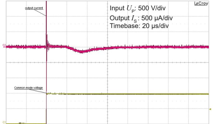
Figure 8: Detail of typical common mode perturbation (1000 V step with 6 kV/ $\mu\text{s}$ ,  $R_M = 100\text{ }\Omega$ )
